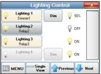
The Lighting Control screen can display up to 4 lights at one time.
