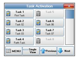
The Navigator Task Activation screen can display up to 8 task buttons at one time. Each task button displays the task number with or without a name.
