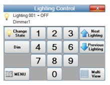
NOTE: Direct number entry is the only way to gain access to to a hidden Light. The Next and Previous buttons skip over hidden Lights.
