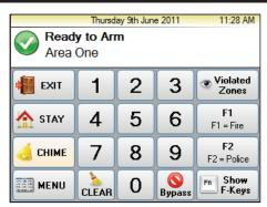
The top line of the Main screen displays the current time and date from the M1 Control. Actual display may vary slightly from that shown.
