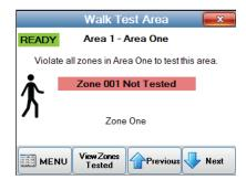
Navigator provides a quick and easy means of walk testing zones without distrurbing your neighbors. This Walk Test option DOES NOT cause any alarm or trouble reports to be transmitted to a Central Station.
